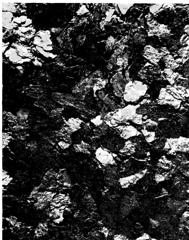
Fig. 8 Pyrolytic graphite crystallite order (model).
