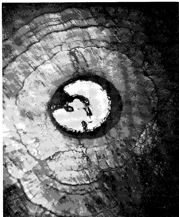
Fig. 5 Defect structures caused by soot inclusions.
